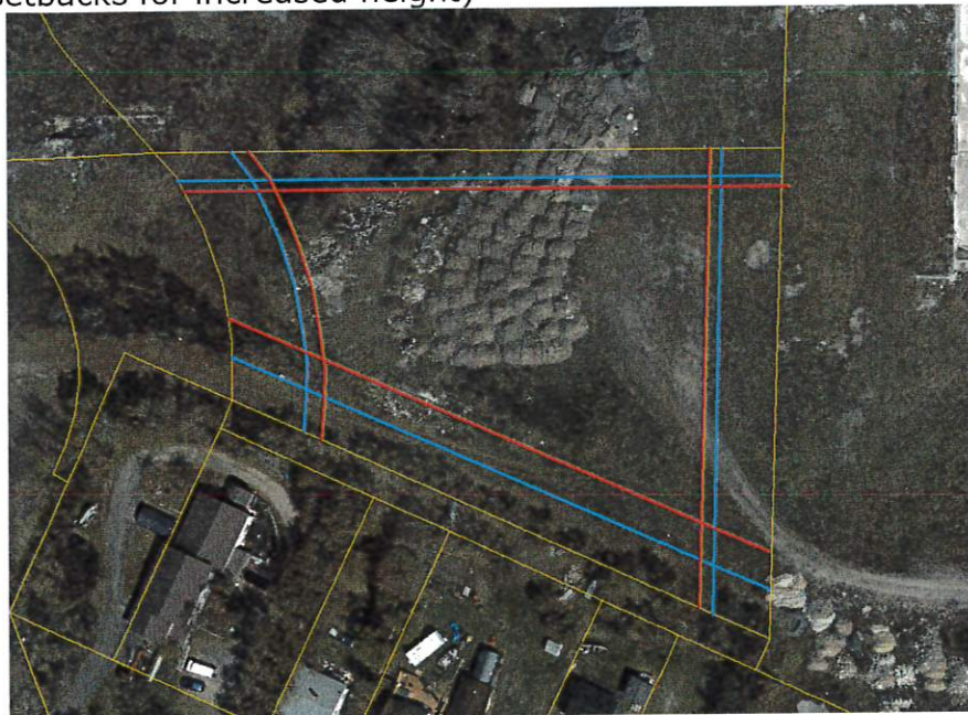
Figure 2. New Building Envelope (blue = minimum setbacks, red = new minimum setbacks for increased height)
